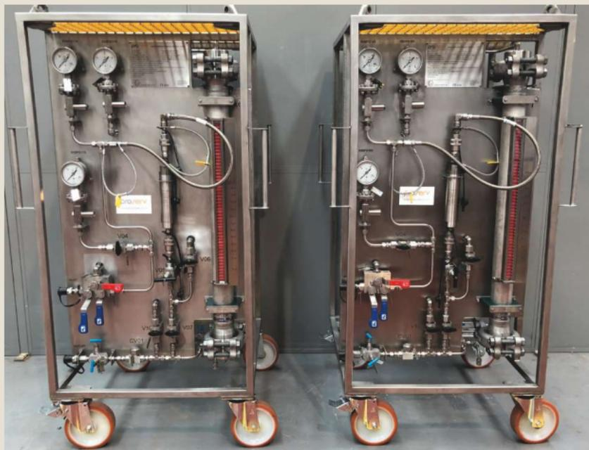
Proserv's sand sampling trolleys represent a portable alternative to open receptacle sand filtration units. (Source: Proserv)
