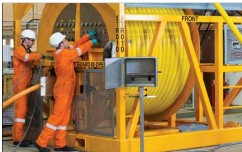
Two Proserv technicians check IWOCS equipment prior to shipping offshore
