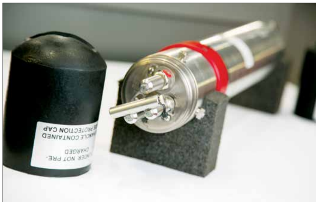
Proserv sampling cylinder showing connection ports
